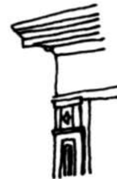
The intersection of Cornice, Fascia and Pilaster on a shop front without Console/Corbel bracket
